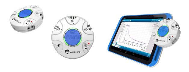
The devices come with their own external sensors, Voltage, Current, Air pressure, pulse, External temperature sensor.
